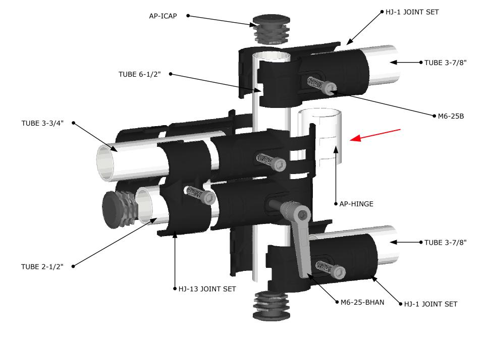
ASSEMBLE ARM MECHANISM, USE CORRESPONDING PARTS AND ENSURE TO TIGHTEN PROPERLY 12-14 Nm
