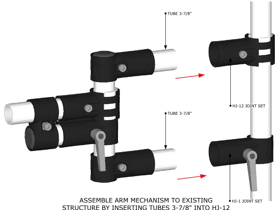
STRUCTURE BY INSERTING TUBES 3-7/8" INTO HJ-12 AND HJ-1 JOINT SETS, TIGHTEN PROPERLY
