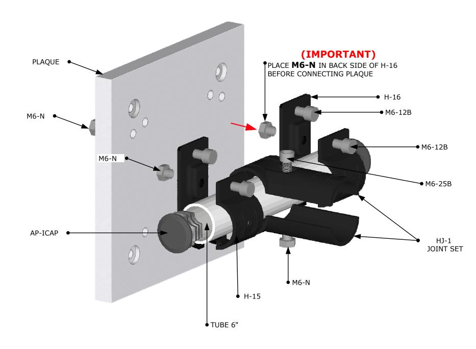
ASSEMBLE USING CORRESPONDING PARTS AND ENSURE TO TIGHTEN PROPERLY 12-14 Nm
