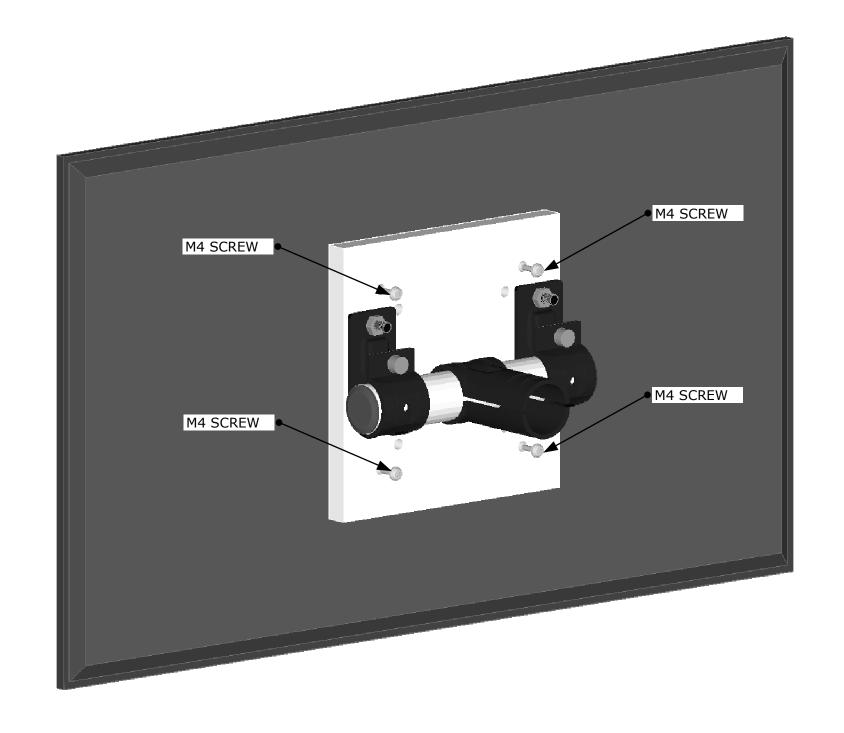
FIX MONITOR TO PLAQUE USING STANDARD M4 SCREWS IN CORRESPONDING OPENINGS (FIND AT HOME-DEPOT)
